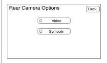
Select the Video screen button. When the Video screen button is highlighted the RVC system is on.
